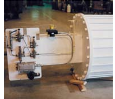
A 42" bore size actuator capable of generating over 200,000 lbs. of force.
