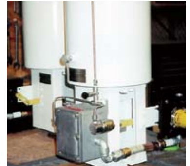
Hydraulic spring return control valve actuators with explosion-proof ATI positioning systems are ready for shipment.
